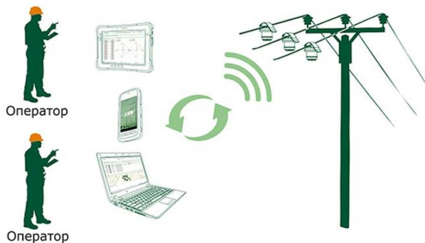
Figure 7. The principle of operation of the ICS via Bluetooth
