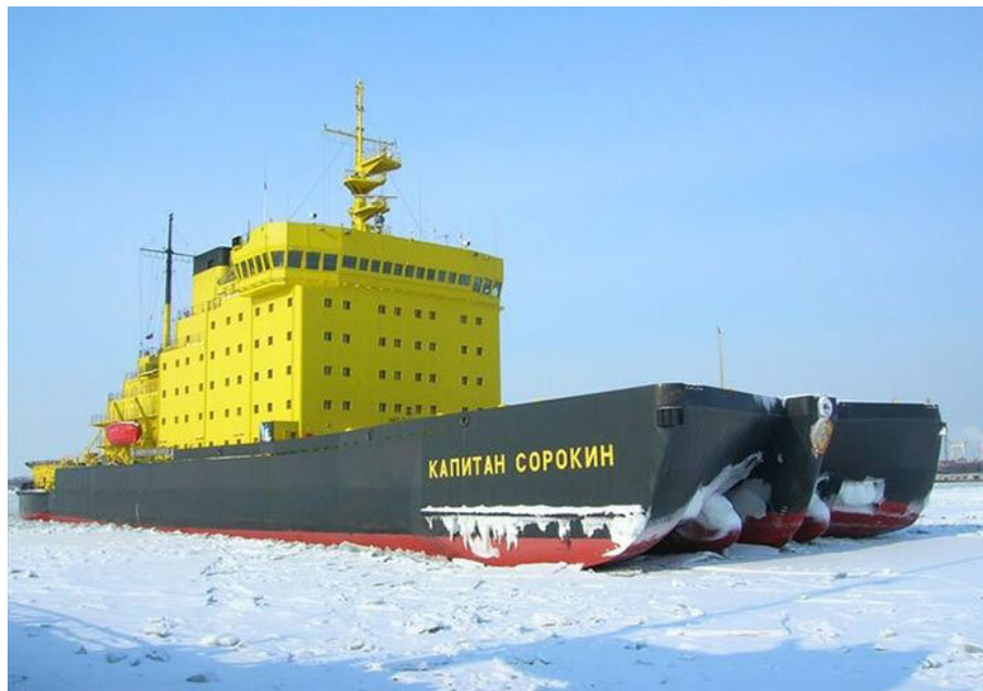
Figure 10 – Icebreaker Kapitan Sorokin with a Thyssen-Waas bow
