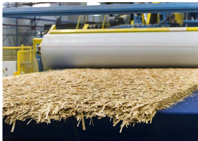
Figure 2 – Pressing of chipboards
