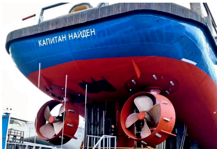
Figure 12 – Mechanical azimuth thrusters
