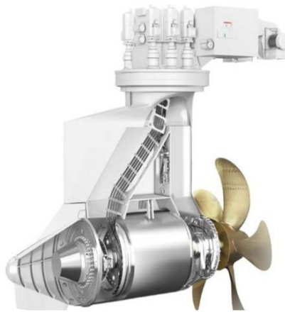
Figure 14 – 3D model of an electric azimuth thruster [12]
