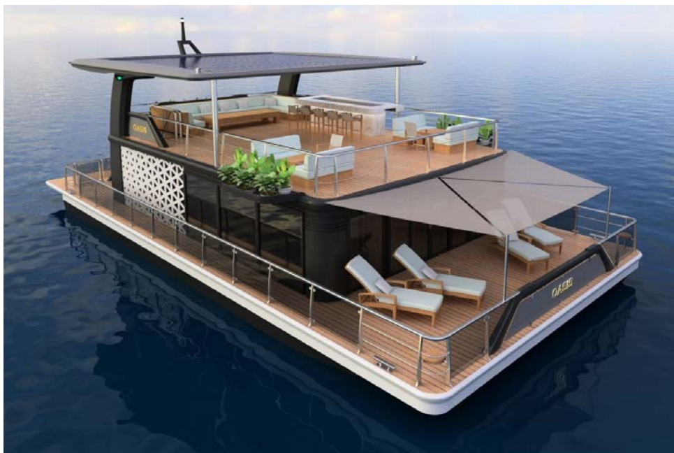
Figure 4 – Presentation rendering of the 3D model of the houseboat
