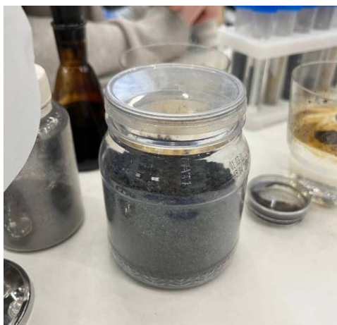
Figure 1 – Thermally expanded graphite
