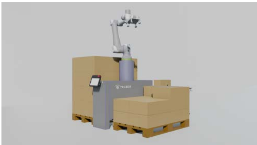
Figure 4 – Robotic palletizing cell with two work areas
