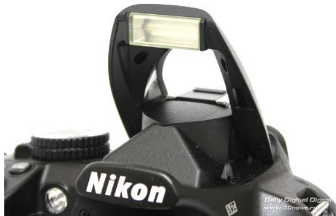
Figure 4. Built-in flash of the Nikon D3000 digital SLR camera
