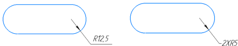
Figure 7. Rule for applying dimensions to identical elements
