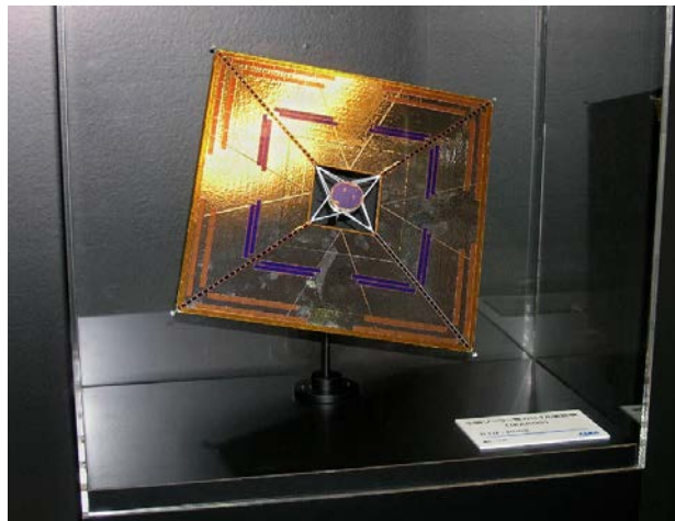
Figure 3. IKAROS is a Japanese spacecraft with a solar sail
