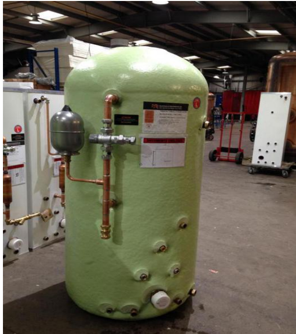
Figure 3. Liquid thermal accumulator
