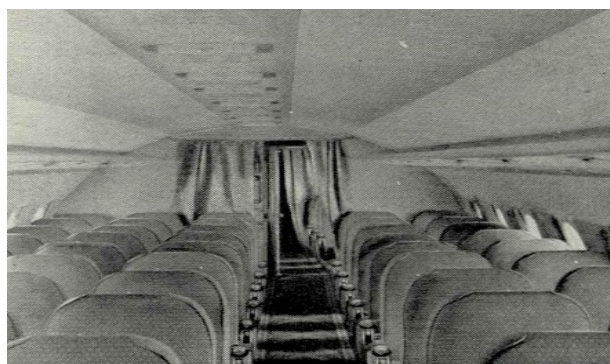
Figure 2 – For the first time, the IL-18 used a panel wall construction with a lightweight laminate covering, foam rubber instead of spring structures for chairs. The IL-18 is the first domestic passenger aircraft equipped with individual lighting and air conditioning (these devices are located in the luggage rack structures)
