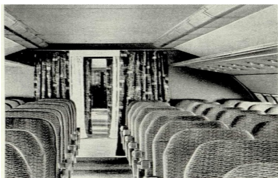
Figure 1 – For the first time, fluorescent lighting, blind luggage racks and rigid blinds moving vertically were used on the IL-62
