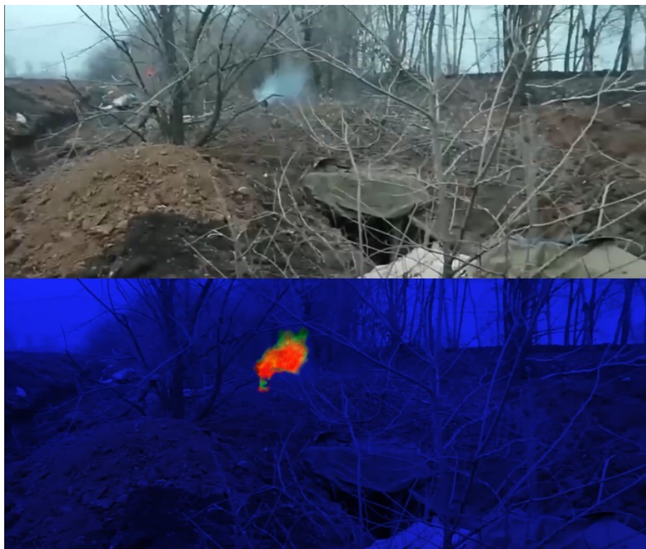
Figure 4. Thermal radiation from the exhaust pipe detected by a thermal imager mounted on a UAV
