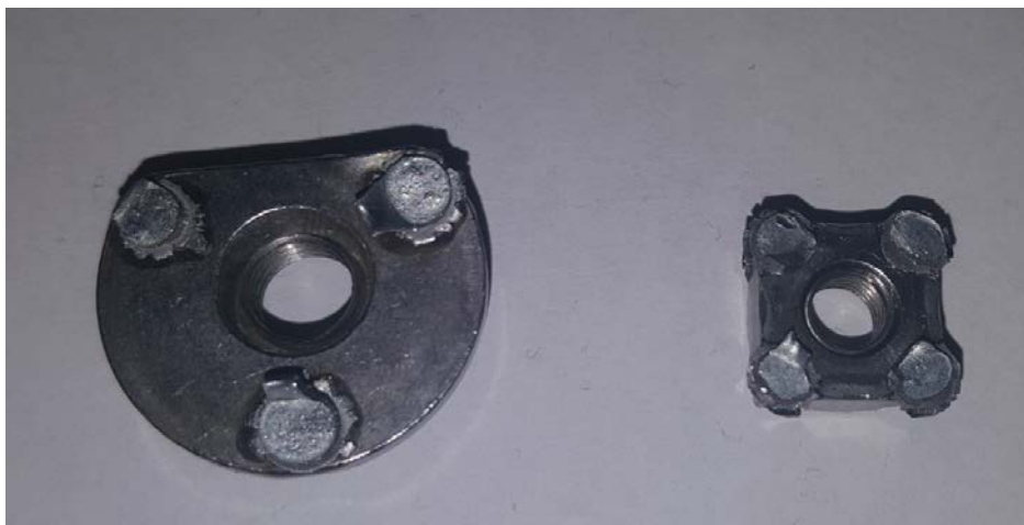
Figure 4. Nuts after the destructive test
