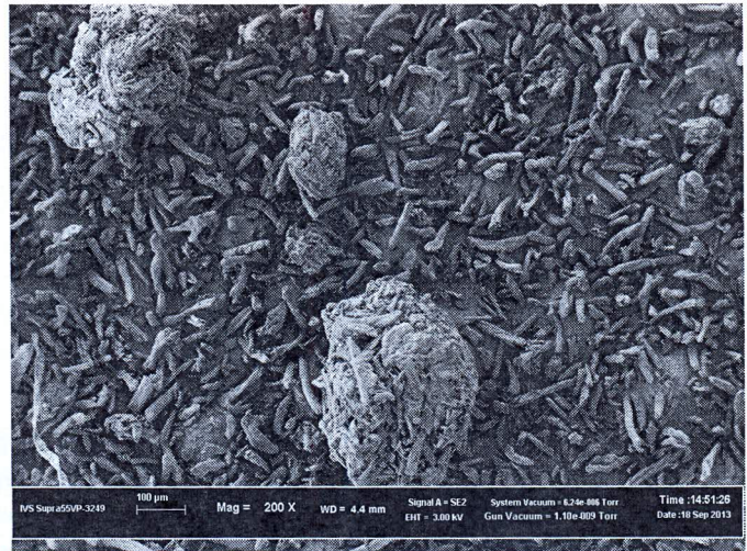
Fig. 1.–SEM image of unscreened microcrystalline cellulose (magnification \times 200 )
